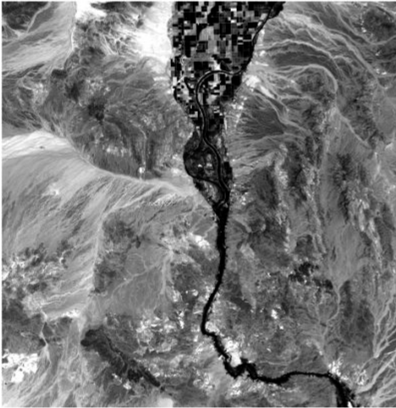
Fig 1.5 An image of part of the lower Colorado River in the southwestern USA. The lightness of the image at any point measures the amount of radiation captured by the satellite's imaging system. Image derived from a public domain SPOT image, courtesy of Alexandria Digital Library, University of California, Santa Barbara.
