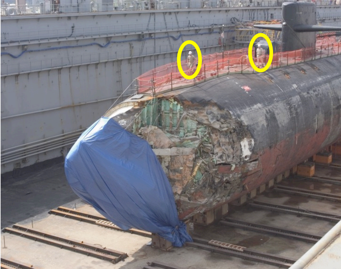
Fig. 1. Photograph of the USS San Francisco in dry dock after the accident (courtesy of David Sandwell, Scripps Institution of Oceanography). Note the men walking within the orange, gated area on top of the submarine for scale.
