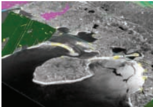
Figure 14. Overlay of a USGS digital orthophotoquad on Buzzards Bay TIN constructed in step 2b of 3-D nautical chart production. Polygons were digitized from the USGS topographic map in figure 13: pink signifies ecologically sensitive areas and yellow identifies barrier beaches, Scraggy Neck portion of Buzzards Bay.
