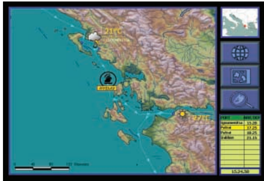
Figure 5. The ship location service interface visually delivers different kinds of data to travelers: real-time ship position, arrival time estimation, and weather information. The authorized version also provides confidential information such as exact ship coordinates and velocity.
