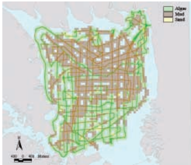
Figure 14. After import into ArcView, the RoxAnn point data was extrapolated using the nearest neighbor algorithm within ArcView Spatial Analyst. This extrapolation was accomplished using a majority classification with a 100-meter cell size. This approach is being tested to determine whether this produces the most accurate results across the entire bay.
