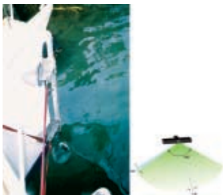
Figure 6. The transducer of the Kongsberg Simrad EM-3000 for transmitting and receiving acoustic beams. The transducer was mounted at the end of a metal pole secured to the port side pontoon of the survey boat and then cabled to the data collection and processing unit within the boat's cabin. The graphic at the right illustrates the swath emitted from standard multibeam transducers.
