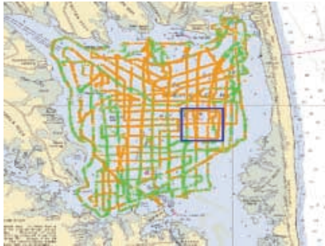
Figure 9. Navigational tracks of the RoxAnn survey color coded by bottom type: orange represents soft bare mud (less than 15 percent algae cover), yellow represents harder mud or sand (less than 15 percent algae), and green represents algae (greater than 15 percent algae). The blue box is the area extrapolated to create the 3-D bathymetric profile in figure 15.
