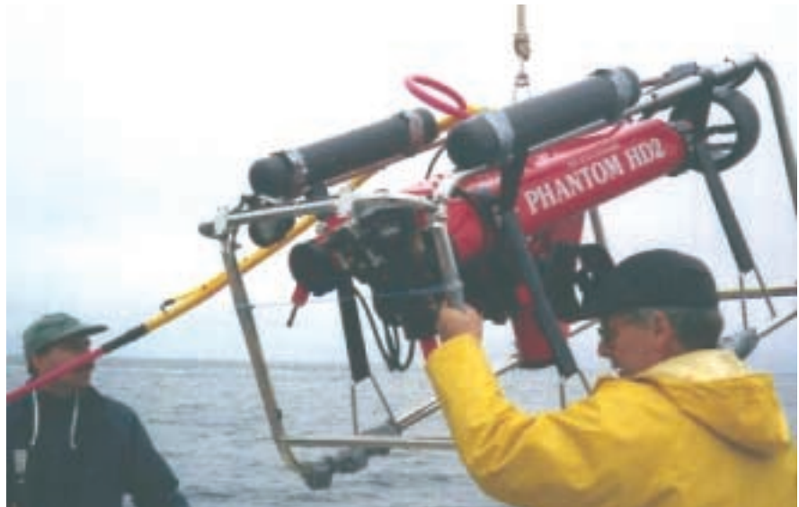
Figure 2. Photograph of the Deep Ocean Engineering Phantom HD2 ROV.
