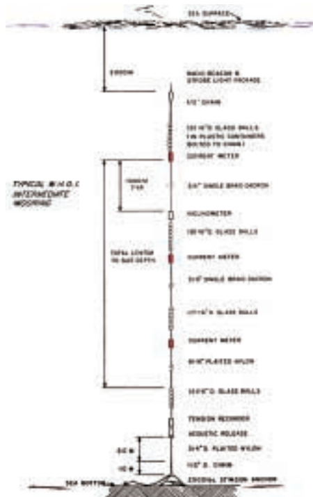
Figure 9. Schematic drawing showing typical oceanographic moored instrument deployment.
