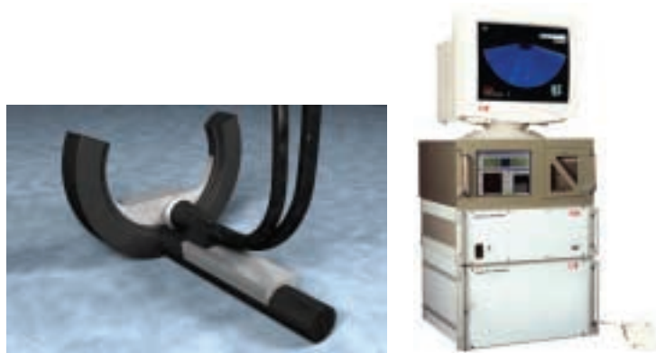
Figure 1. Photographs of typical components in a multibeam echosounding system: (left) transducer head used to emit multiple sound pulses; (right) data collection and processing unit with receiver array and on-screen display of measurements in real time. Reprinted by permission of RESON A/S Underwater Acoustics ( www.reson.com ).
